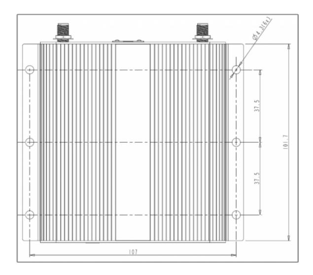
The 6 mounting holes in the CloudGate housing allow mounting on a wall or on a DIN rail. See the details in the "Mounting" section of the CloudGate Installation Guide.
